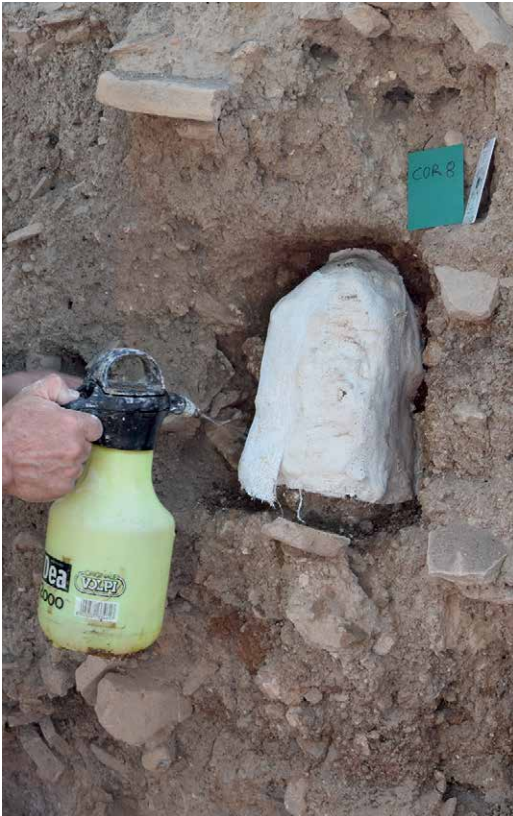
↑ Figure 2. Sampling for micromorphology in a stony soil profile using a gypsum bandage (Photo by S. Khamnueva-Wendt; image modified).
