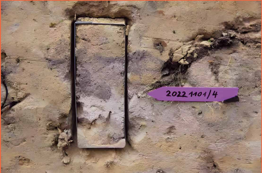
↑ Taking a block sample for the micromorphology of a sod that was used to build a fortification (Vecračina, Latvia) (Photo by J. Schneeweiß; image modified).
