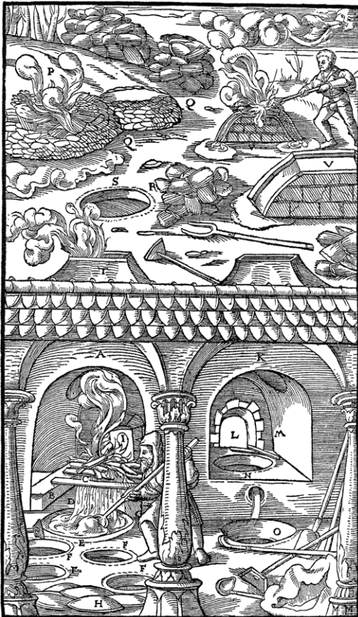
← Figure 3. Different types of furnaces used for lead smelting (Source: Agricola 1556. De Re Metallica ; image modified).
