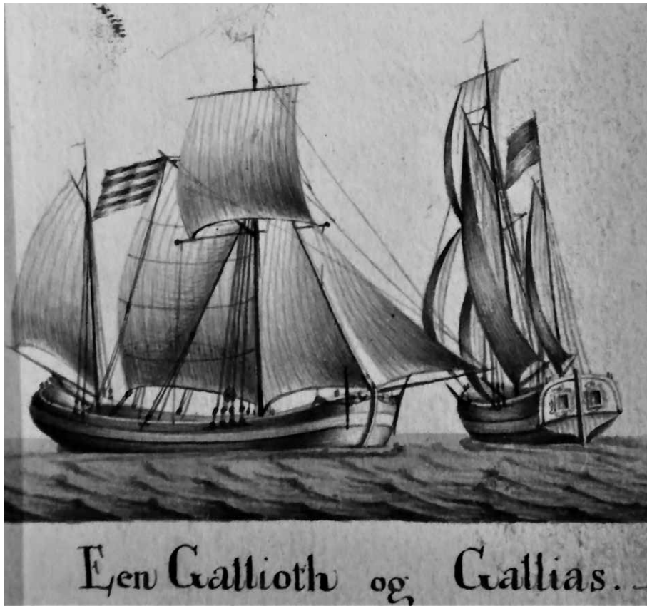
Fig. 4.6. The related types, the galjoot and galeas. The Stibolt Brothers 1763. The Danish Maritime Museum.
