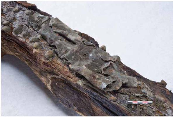
Figure 5. Napoli E. Detail of lead sheathing covering the keel fragment L9 (Photo P. Groscaux AMU, CNRS, CCJ, courtesy of Superintendency of Naples).
