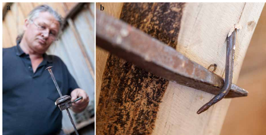
Figure 7. The copper nails: a) coppersmith Igor Shteiman with a newly made nail; and b) double clenching a nail over the inside surface of a frame (Photo A. Efremov).
