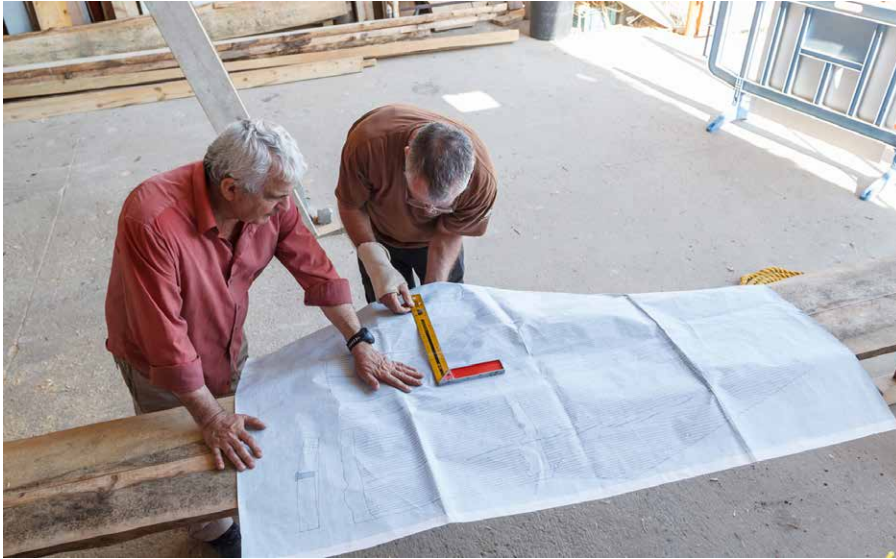
Figure 2. Y. Kahanov and carpenter Avihay Ismann copying an archaeological drawing onto a plank (Photo A. Efremov).
