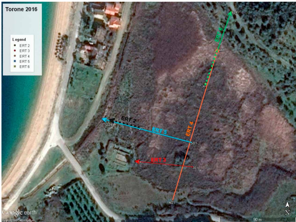
Figure 10. The ERT arrays laid out in 2016 (Republished, with kind permission, from Meditarch , 2016, 28-29. Mapping by G. Tsokas and P. Tsourlos, using Google Earth 2016 CNES/Astrium).
