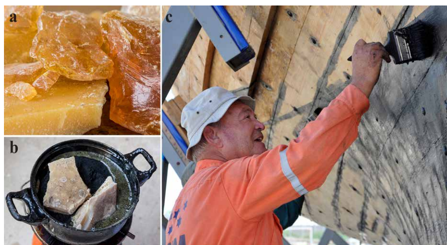
Figure 8. Coating the hull: a) beeswax and pine resin (Photo A. Efremov); b) the boiling mixture (Photo A. Efremov); and c) Zeev Blass painting the underside of the hull with the black mixture (Photo John Tresman).
