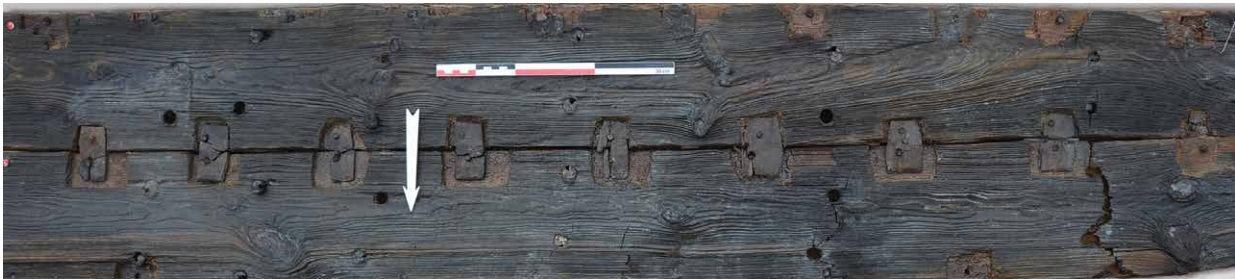
Figure 7. Two adjacent strakes on the starboard side with the mortises opened to reveal the tenons (Copyright Marie-Pierre Jézégou).
