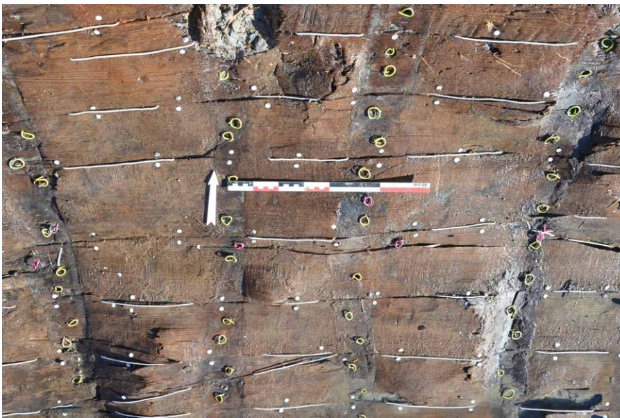
Figure 9. Frame planking fastening on the starboard side. The pink rings are nails; the yellow ones are treenails (Copyright: Julie Labussière).
