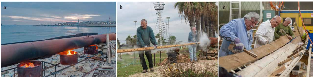
Figure 3. Bending the hull planks: a) the timber boiler in operation, with the Old City of Akko in the background (Photo A. Efremov); b) the hot plank is taken to the hull (Photo A. Hillman); and c) installing a plank using temporary tenons and clamps (Photo A. Efremov).
