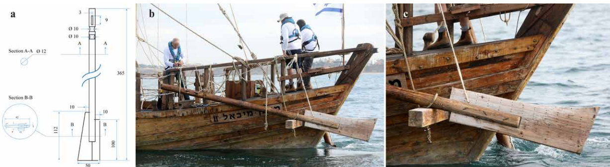
Figure 12. The quarter-rudders: a) a schema (Drawing Ofer Zahavi); b) the port rudder and its attachment to the hull; and c) a closer view of the port rudder (Photo Nimrod Gluckman).
