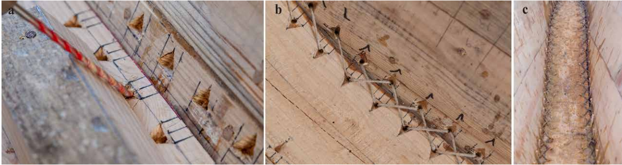
Figure 5. Sewing of the hull: a) drilling the sewing holes from inside the hull at an angle of 45° to the surface of the knee; b) the cord threaded through the sewing holes; and c) the bow knee (Photo A. Efremov).
