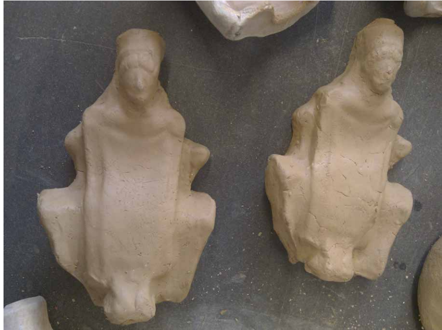
Figure 3.2: If the clay is too dry, this may result in cracks on the surface after being pressed into the mould.
