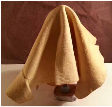
Figure 5.2-9a. 0 = Very soft handle with lofty fibres, stretch in all directions and a limp drape. Bends in two dimensions and forms folds. Similar in drape to a medium weight T-shirt.
