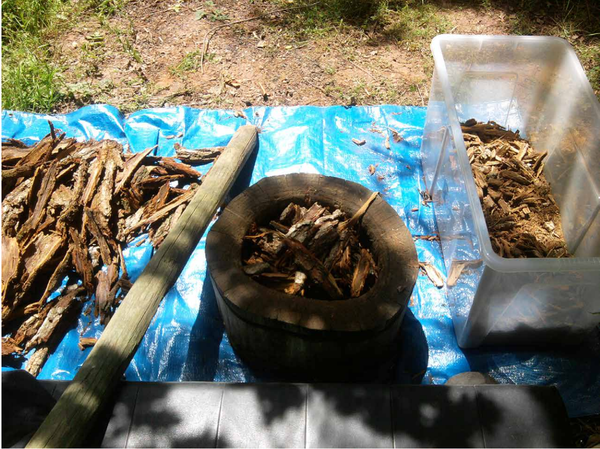
Figure 4.4-1a and 1b. A- Oak bark being processed in a large wooden mortar. The large strips as they were pulled from the tree (left hand side of photo A), B- the size after crushing.
