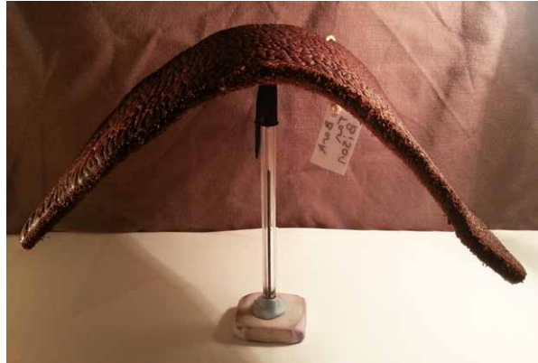
Figure 5.2-9e. 4 = Moderate bendability with no loft, no stretch, a stiff drape and in some cases a cardboard sound when flexed. Forms a very open rounded U shape and has only unidirectional bend. Similar in drape to very heavy canvas.
