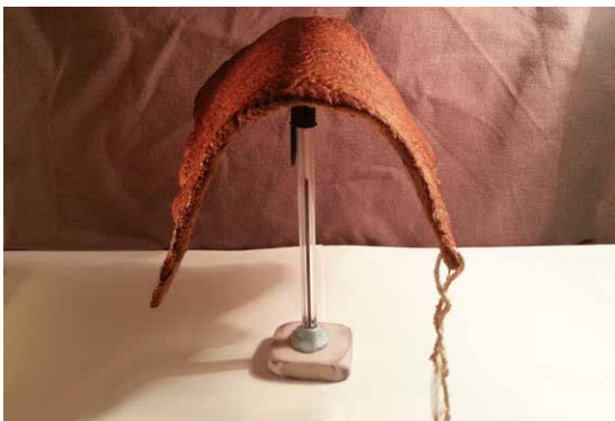
Figure 5.2-9d. 3 = Flexible but with little loft, little to no stretch, a stiff drape and in some cases a papery sound when rustled. Forms an open U shape and has only unidirectional bend. Similar in drape to medium duck canvas.
