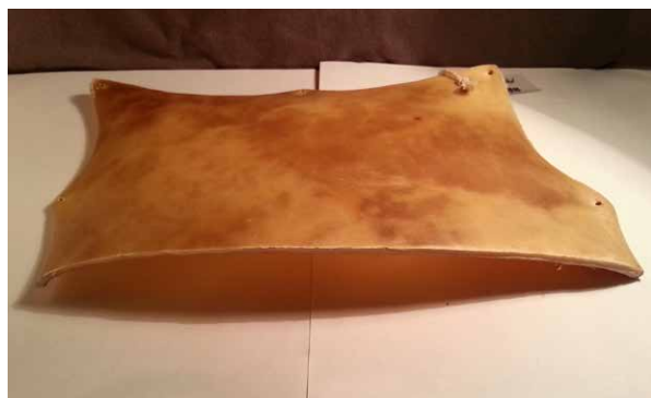
Figure 5.2-9g. 6 = Very hard, no bendability but may flex slightly. A feel equivalent to a piece of 1/4 inch (4mm) plywood.
