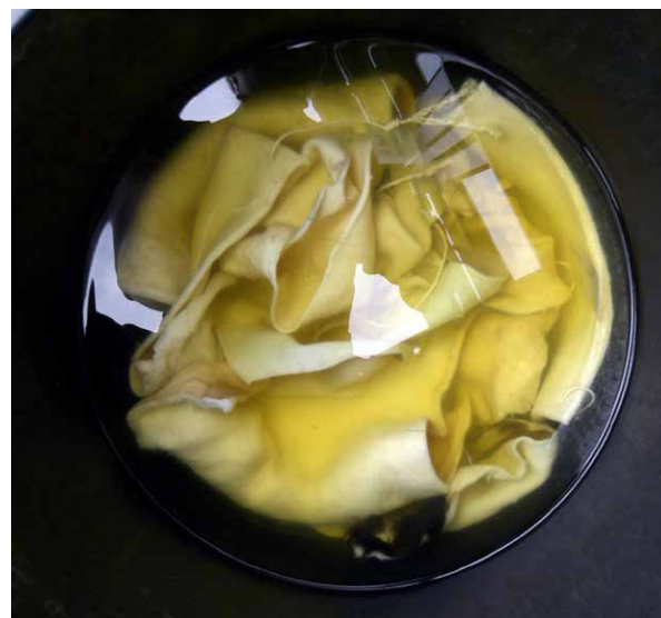
Figure 4.6-1. Hair-off samples soaking in the urine solution. (Looking down into the solution).
