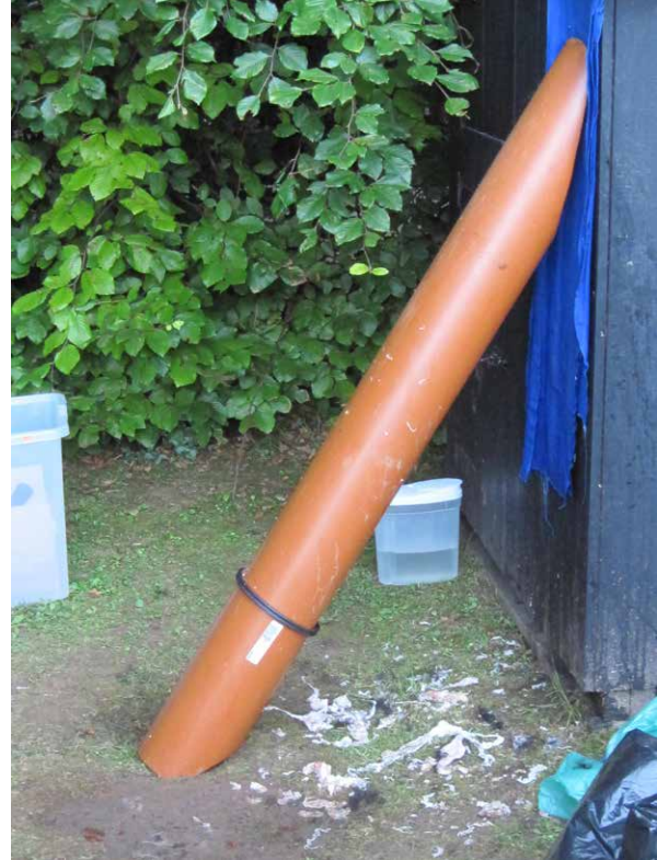
Figure. 4.2-2. Plastic tanner's beam, which can be used as a 'Pull' or 'Push' beam.
