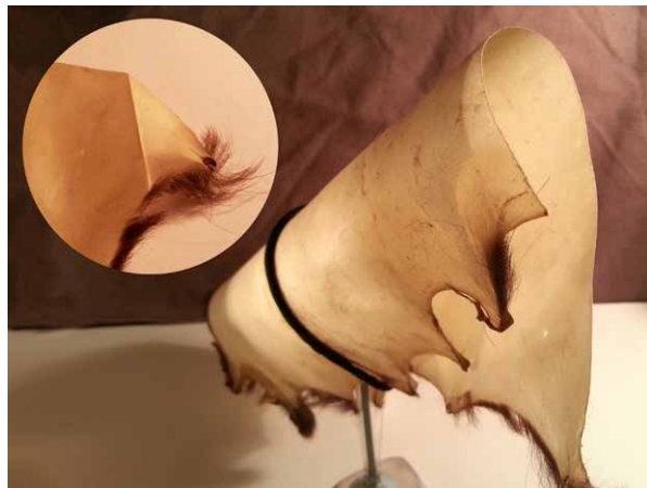
Figure 5.2-9f. 5 = Hard, cracks or splits when bent or permanently creases, no drape. Similar to the feel of post card paper. Inset illustrates a permanent crease.
